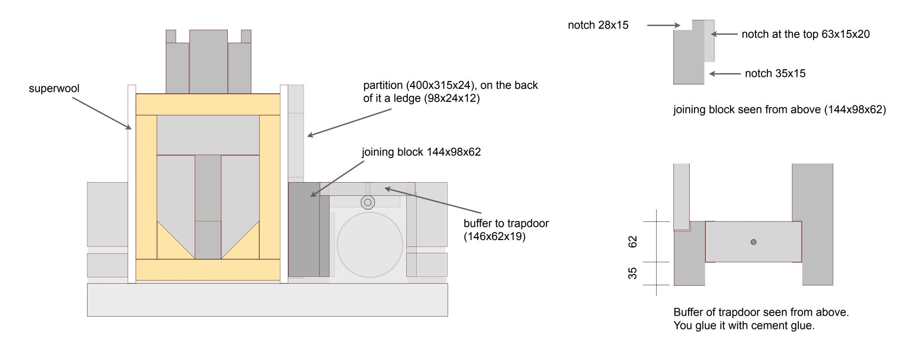
08. Installing the core, joining block and partition, buffer to trapdoor
