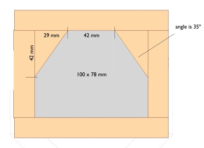
Top of firebox (solid refractory concrete). Height of moulds: 32 mm
