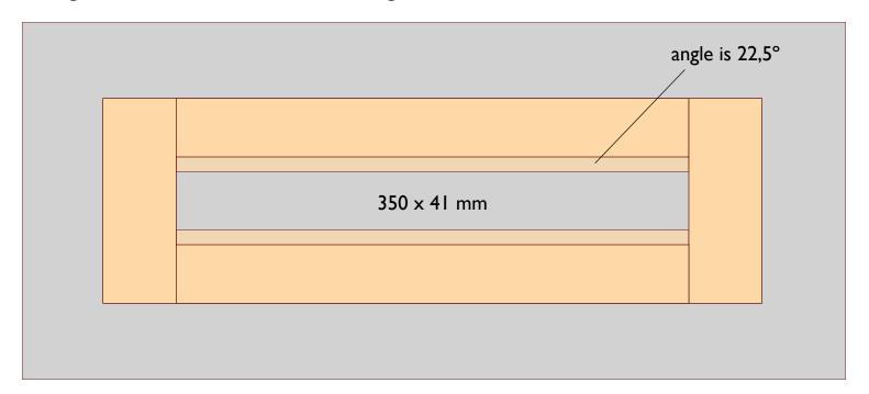
Heel (insulating refractory concrete). Height = 24 mm. After hardening, the heel is adjusted with a grinder to make it fit in the riser.
