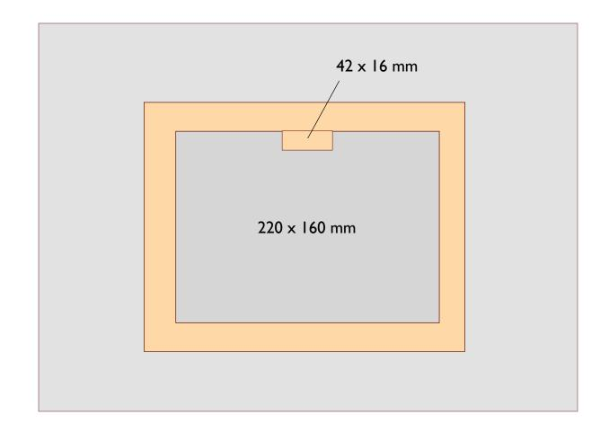
Port (solid refractory concrete). Height of moulds: 32 mm
